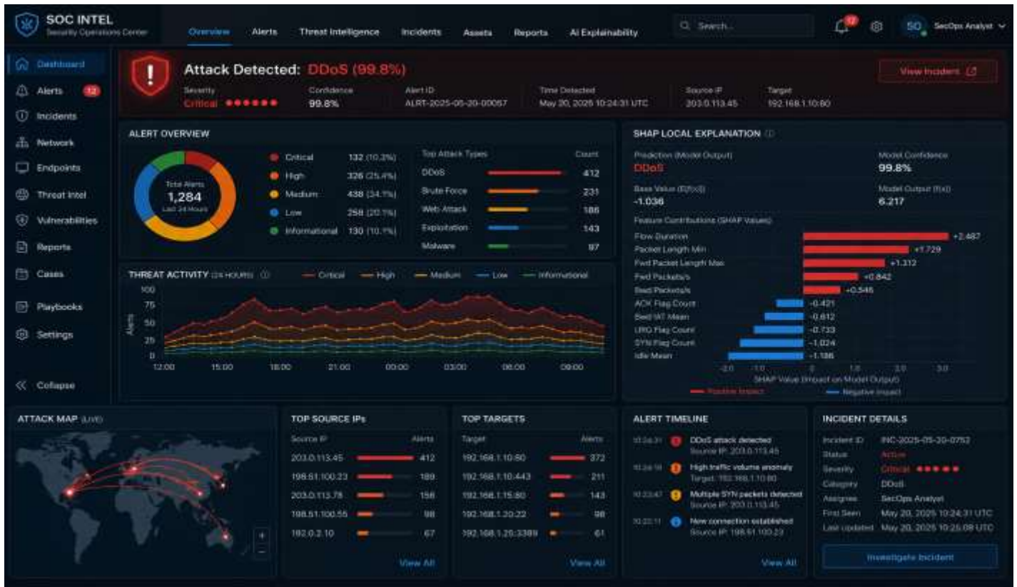
Figure 3: A model of the Interpretable Dashboard and Analysis in Security Operations Centers (SOCs) based on Shabli Added Values (SHAPs). The visual panel illustrates the contributions of different network features to the hybrid modeling of its final decision to classify the flow as a threat, where features marked in red positively contribute to raising the likelihood of an attack, while blue features pull the decision toward the normal state, giving the security analyst immediate explanation and scientific justification to support measures Rapid defensiveness and reduces the accumulation of unexplained alarms (Khan et al., 2025).
